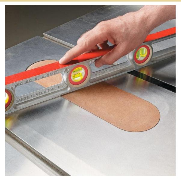
Press the plate into the opening until it's flush with the table. I use a straightedge, like the level shown here. The paste wax prevents the glue from sticking to the tabs. But it sticks to the insert plate to keep it level. In just a few seconds, I have a flush insert plate that I can use over and over.
