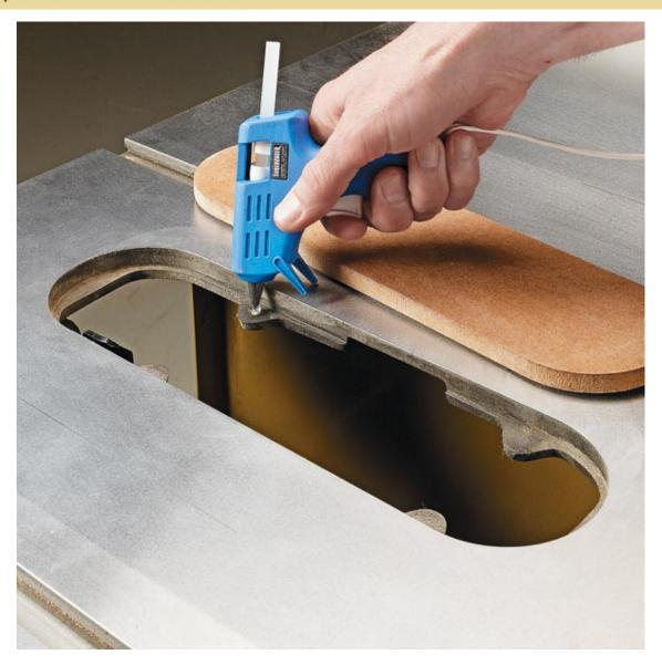
Leveling a shop-made insert plate on your table saw can be a time-consuming process. But I found a quick and easy way to tackle this chore using a hot-melt glue gun and some paste wax.
