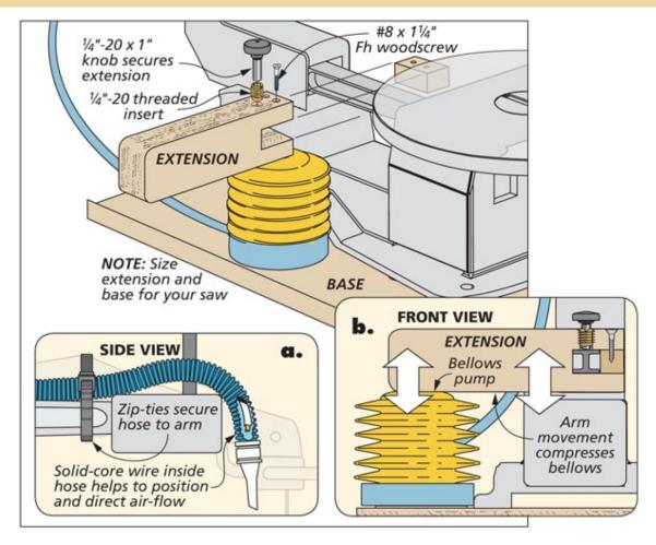
The pump is attached to a plywood base next to the saw. An extension arm, secured to the lower arm of my scroll saw, fits over the top of the pump. When operating the saw, the oscillating action of the arm moves the bellows and supplies puffs of air to keep the workpiece clear.
