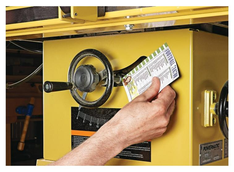
To make dust collection more efficient, John Cusimano of Lansdale, Pennsylvania, seals the slot in the front of his table saw with a large sheet magnet.
