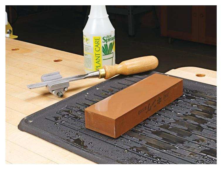
John Doyle of Ankeny, Iowa, uses water stones to sharpen most of the edge tools in his shop. But the process tends to get water all over his workbench. To keep things cleaner, he uses an inexpensive rubber car mat to contain the mess.
