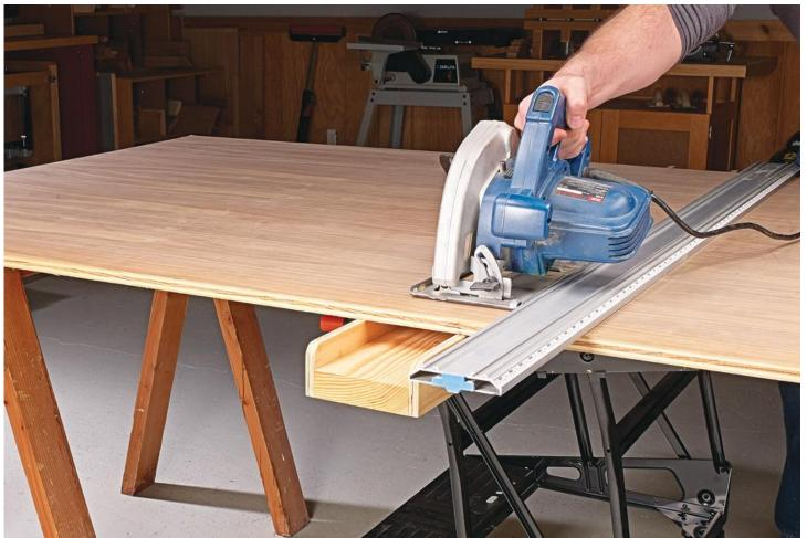
When it comes to breaking down sheet goods, there's certainly no shortage of ways to complete the task. But I was looking for a way that would utilize my Workmate bench without cutting into the work surface. What I devised is the setup you see above. This method uses a C-channel made from a 2x6 for the base and some plywood scraps that act as risers. The risers are attached to the base with screws. I sized my pieces so they're a couple feet longer than my Workmate.
