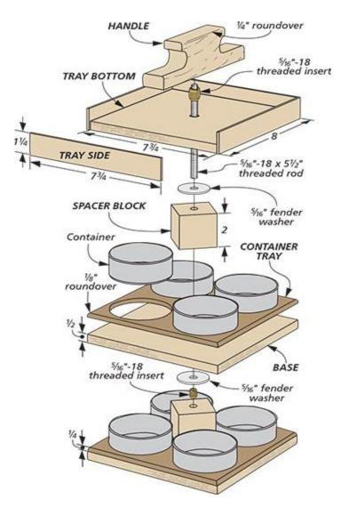
Begin by cutting two pieces of hardboard to the dimensions shown for the container trays. Using a circle cutter at the drill press works great to make the four holes in each of the pieces. The base pieces are cut from plywood and are attached to the container trays with glue. I eased the top edge of the hardboard trays with a roundover bit. The two spacer blocks are now cut to size and glued to the container trays, as shown in detail 'a.'
