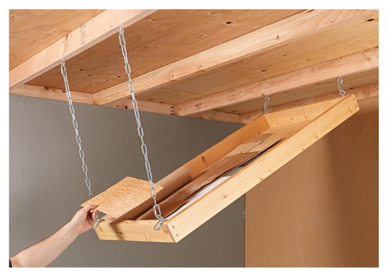
My small shop doesn't have much room for storage, especially when it comes to delicate sheets of veneer and various lightweight items that are easily damaged or misplaced. To solve this storage problem, I made this shallow tray that's mounted to the rafters in the ceiling.
