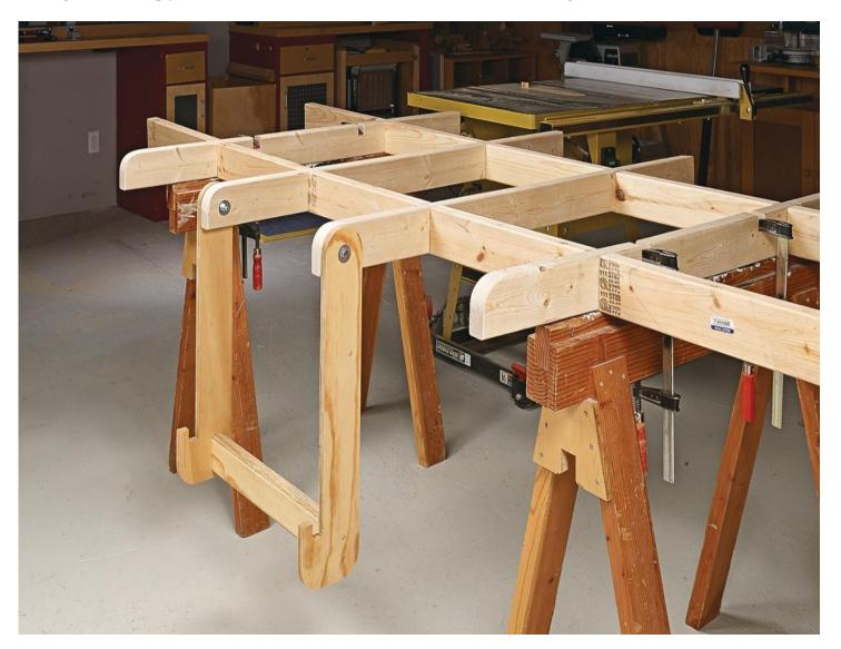
Last year, I built a knock-down cutting table. This quick-to-assemble table clamps to a couple of saw horses and is perfect for breaking down sheet goods. To make the table even more user-friendly, I added the swing arm lift you see here to assist in loading large sheets of plywood onto the table.
