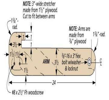
The plywood arms have a notch cut on one end which was easily accomplished with a jigsaw. A two-layer plywood stretcher connects the two arms. The arms are attached to the knock-down table with bolts, washers, and lock nuts.
