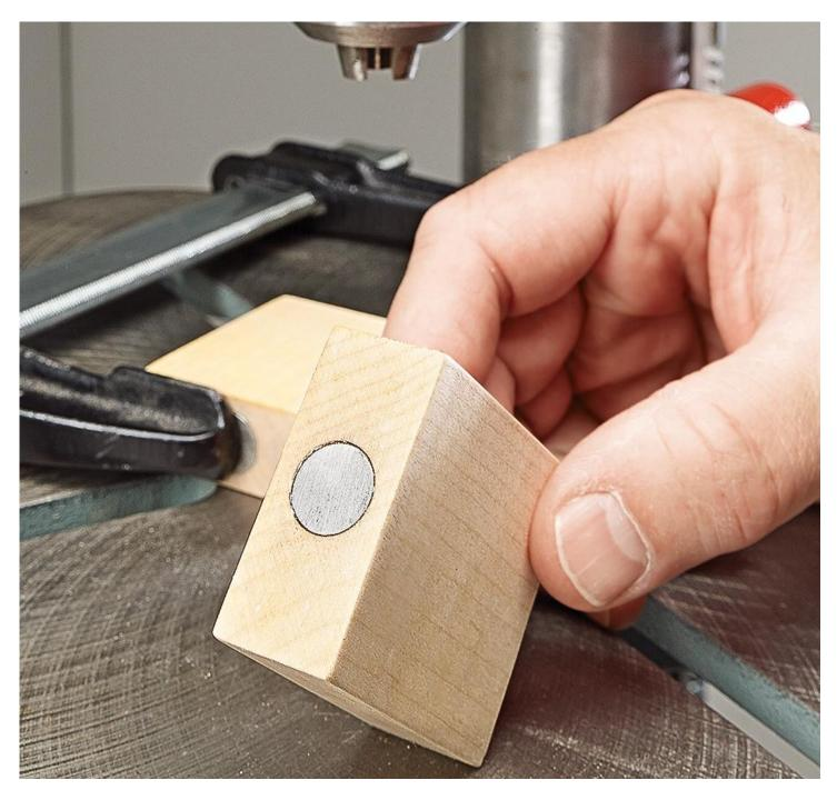
So you don't have to fumble holding the block and clamp, a rare-earth magnet is recessed in the end of the block, as shown in the photo above. I like to keep several sizes of blocks by my drill press to accommodate varying sizes of items that may need to be clamped to the table. Simply stick the magnet end of the block to the underside of the table and clamp it in place.
