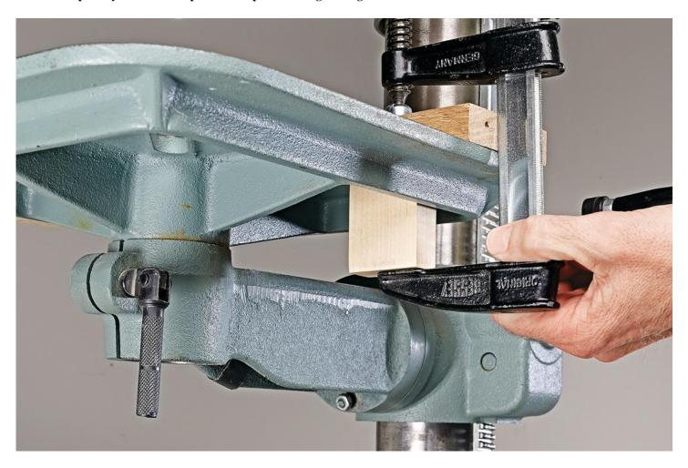
Because of the cast webbing on the underside of my drill press table, it can be difficult to clamp a fence or workpiece to the table. To solve this problem, I made these simple clamping blocks. The blocks, along with a regular, F-style bar clamp, allow you to "step over" the webbing to secure items to the table.
