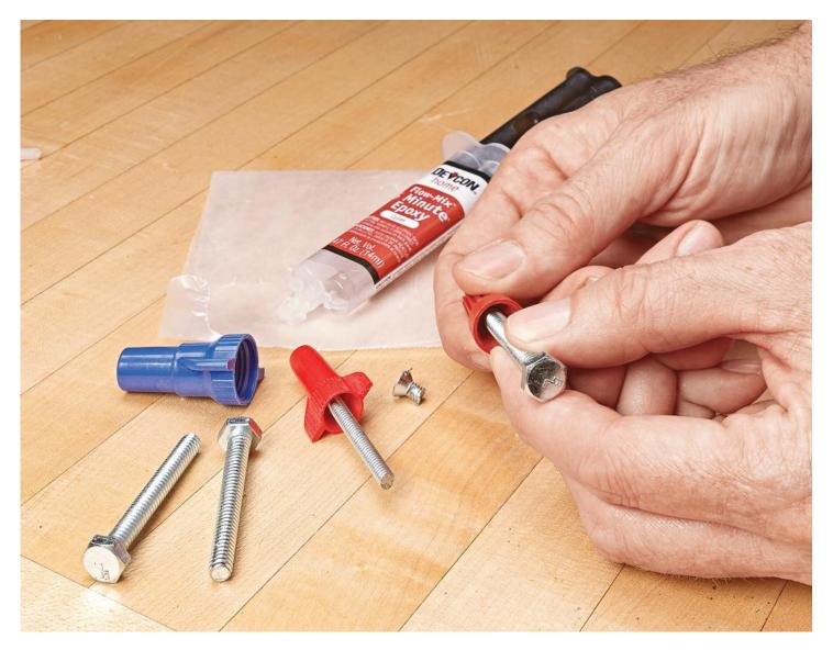
Whenever he needs an odd-sized thumbscrew, Philip Jacobs of Saint Paul, Minnesota, simply makes his own. He threads a bolt into a wire connector as far as it will go and fills the void with epoxy. After the epoxy cures, he cuts off the bolt head.
