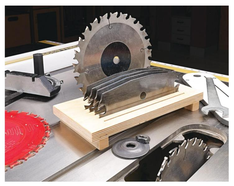
To make the caddy, I started with an extra-long piece of plywood and raised the spinning saw blades into the base in order to cut the slots for blades and chippers. To do this, you'll want to use the saw's rip fence to position each slot, and clamp the plywood blank securely to the front and back of the saw table for each cut. Once that's done, you can simply cut the base to length, attach the hardwood cleats, and set all your blades and chippers in place.
