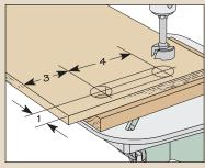
**Set the Boundary.** You can use a 1" Forstner bit to cut a hole at each end of the handle.
