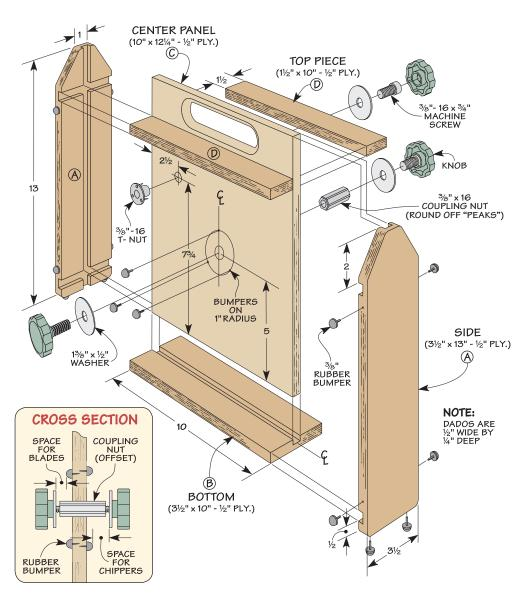
up more space than the scoring blades, the coupling nut is offset to the chipper side of the case, as you can see in the Cross Section above. Epoxy will hold both the Tnut and the coupling nut in place. I also added knobs to the cap screws for the coupling nut to make them easier to tighten and loosen.
