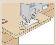
**Remove the Waste.** Then use a jig saw to remove the waste for the handle in the center panel.
