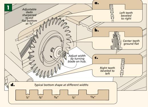
dadoes is that at most settings they don't cut a flat bottom. The better ones are specially sharpened (Fig. 1) to cut flat at a specific width (usually  $\frac{1}{2}$ " or  $\frac{3}{4}$ "), but at any other width you're out of luck. In Fig. 1d, you can see how the shape of the bottom changes with the width of the cut.
