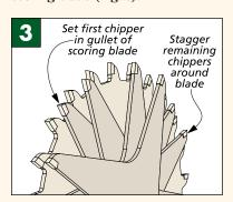
Now as more chippers are added, they should be staggered to balance the blade (Fig. 3). Then after the outer scoring blade is added, I make sure that nothing shifts when I tighten down the arbor nut.
