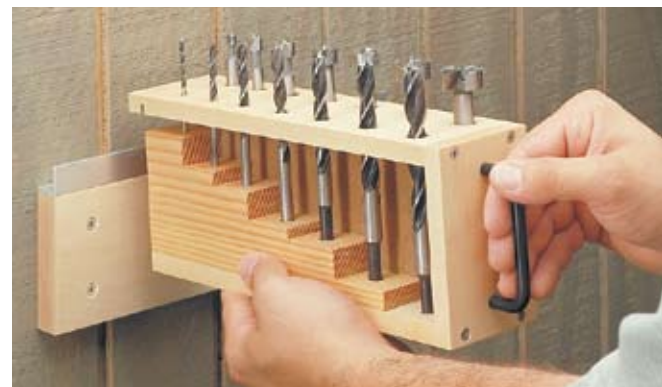
▲ Removeable Hangers. Each hanger hooks onto a metal rail attached to a wall-mounted cleat. To drill a hole in a project at the bench (or around the house), simply lift the hanger off the rail and take the bits with you.
