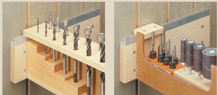
▲ Cleat. A two-part cleat that's made up of a hardwood mounting plate and a metal rail lets you hang each of the racks (left) and bins (right) on the wall. Just be sure to anchor the cleat securely to the wall.
