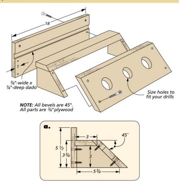
The dock is made entirely from <sup>3</sup>/<sub>4</sub>' plywood. To build it, I drilled a series of holes in an angled shelf front. The holes are sized to accept the chuck on each drill that I own. The shelf front is supported by a pair of braces and a small top. These are attached to a plywood back that hangs on the wall.
