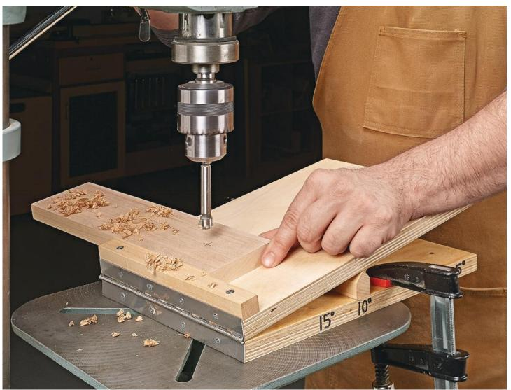
When drilling angled holes, I used to just prop up the workpiece with scrap wood on the drill press table and eyeball the angle until it looked right. Then I was building a complicated coat rack with multiple pegs, and I realized I had a problem. To improve the accuracy and consistency of my holes, I made this adjustable angle support which has proven useful for many projects.
