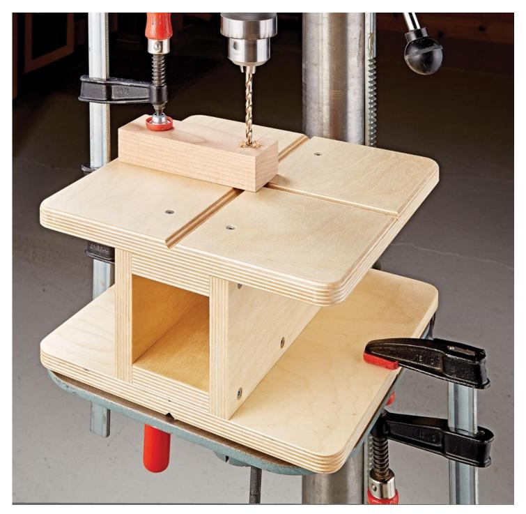
I do a lot of metalworking in my shop. This often leaves my drill press table oily and covered in metal shavings. To use my drill press for woodworking, I wanted a quick-change option that would give me a clean work surface without going to the trouble of building a large auxiliary table.
