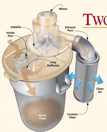
▲ How it Works. Dust is drawn directly into the garbage can, where heavy particles settle. Fine dust is captured in the canister filter.
