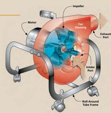
How it Works. Both heavy chips and fine dust are drawn directly through the impeller. A single bag functions as both chip collector and dust filter on units such as this.
