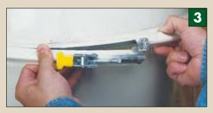
▲ Using Suction to Connect. To reattach the cone after installing the clean filter, first make sure all of the blast gates are closed. Then turn the cyclone on and let the suction draw the cone tight against the barrel (Fig. 2). The suction will hold the cone tight against the bottom of the barrel and allow you to use both hands to reattach the snap ring (Fig. 3).
