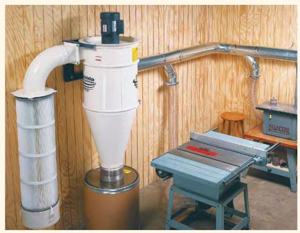
Although often configured as a central system, as shown here, cyclones can be used as portable systems.
