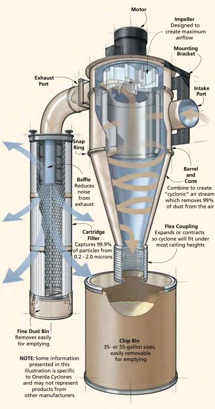
▲ **How It Works.** Debris enters the barrel and is separated in a "cyclonic" stream of air. Large dust particles and chips fall into the bin and finer dust is trapped in the cartridge filter.
