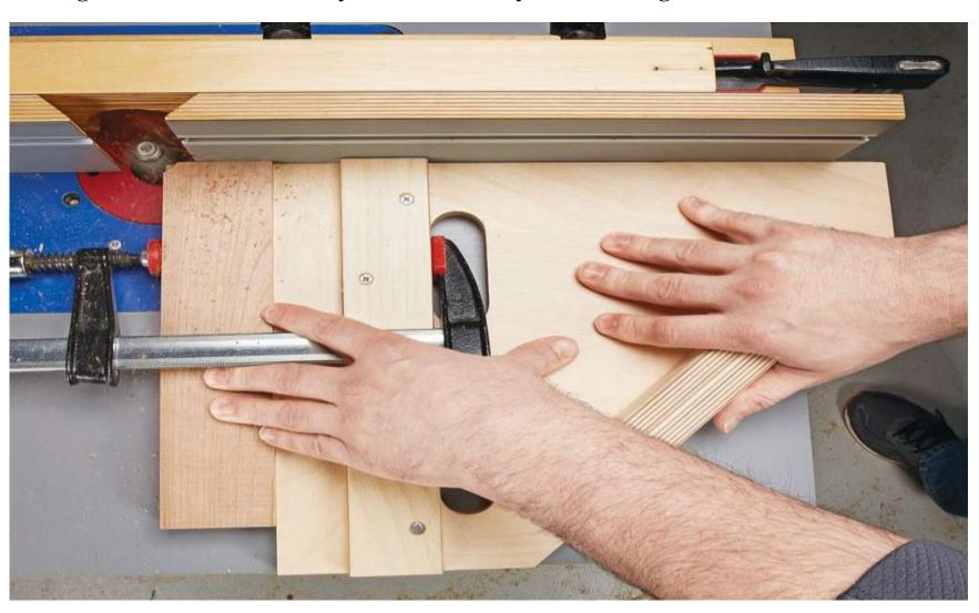
Recently, I was working on a project that required cope and stick doors. To help me rout the end grain cleanly and quickly, I built the jig shown here.
