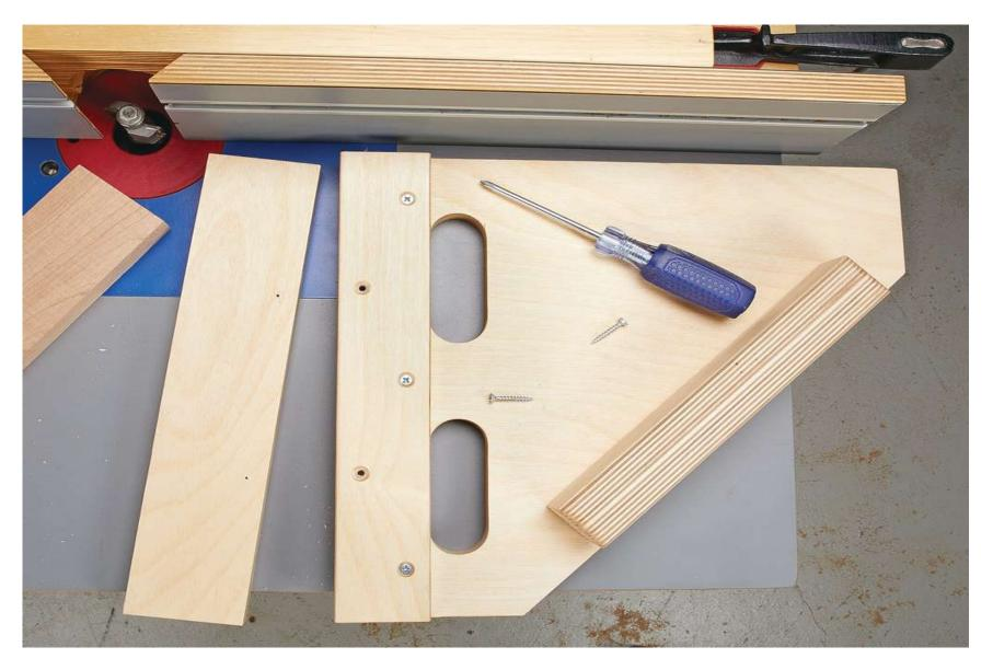
The sacrificial backerboard is held in place with a cleat and screws. This allows it to be easily replaced.
