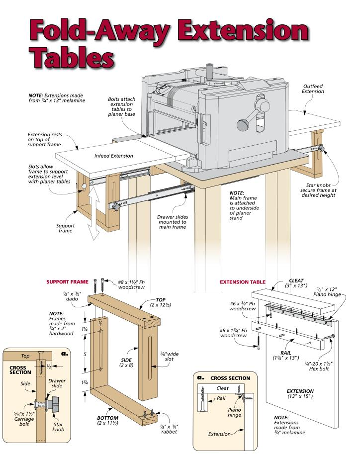
I wanted to extend the short tables on my thickness planer, and adding extensions would be a great way to increase the surface area of the planer bed for working with long boards. But I don't have room in my small shop for a large, permanent setup. So, I came up with the space-saving solution you see here.
