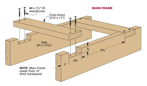
extensions simply rest on top of the frames when extended. Slots in the frame sides allow you to level the extensions.
