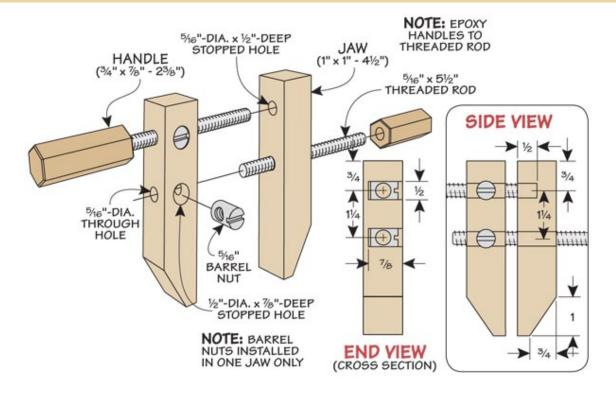
The drawing shows what you'll need to put a clamp together. Threaded rod and barrel nuts perform the work with shop-made handles as a final touch. As you can see, the upper hole in one of the jaws is stopped. This allows the rod to expand the jaws. Even though these clamps don't open and close the same way as traditional handscréws, it doesn't take long to get the hang of it.
