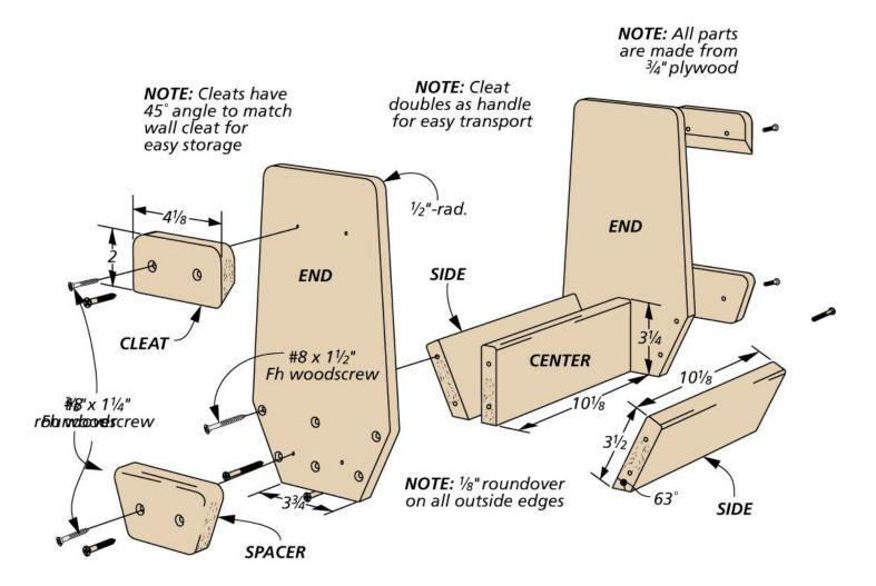
The design of the caddy allows it to hold most sizes of handscrews. Plus, it's small enough to carry right to my workbench, using the angled cleats as handles. And the open bottom ensures that it won't fill up with sawdust.
