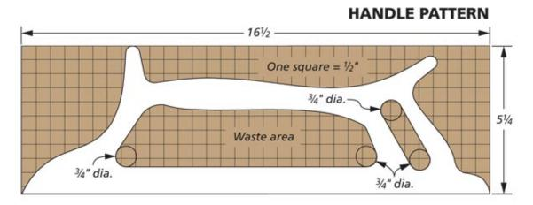
You can shape the handle using the pattern shown here. I cut the outside out first. And then I cut the out the hand grip at the back and the handle in the center. To get smooth curves, you can drill out the corners of the waste with a Forstner bit.
