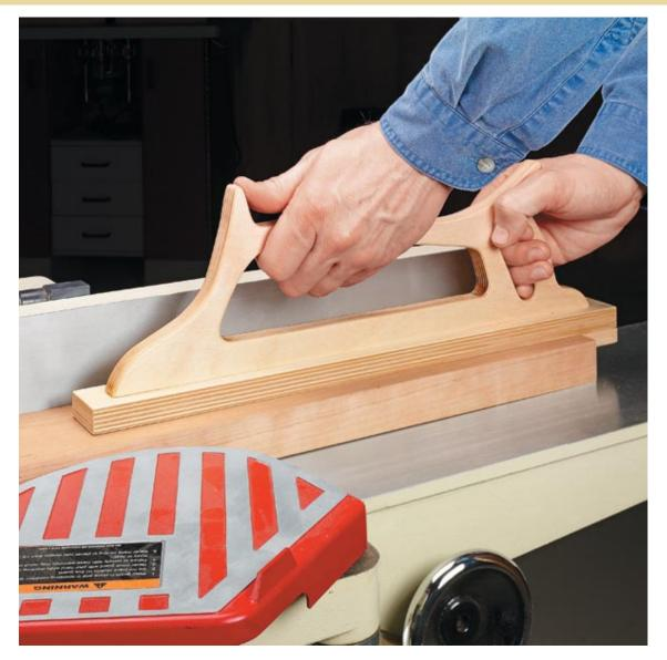
I've found that a push block that both pushes and holds down the workpiece on the jointer isn't easy to find. So I decided to make my own.
