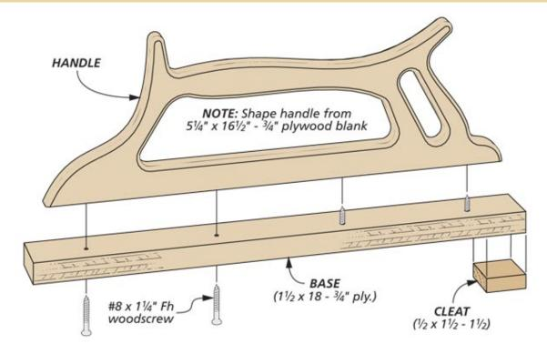
This drawing shows how the push block is built from just three parts: a handle, a base, and a cleat. The base is attached to the handle with screws countersunk in the base. The cleat is simply glued on.
