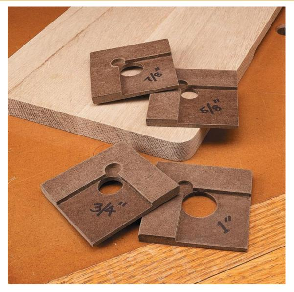
After gluing the two layers, use a marker to label the diameter. I made several templates to match radii that I use most often.
