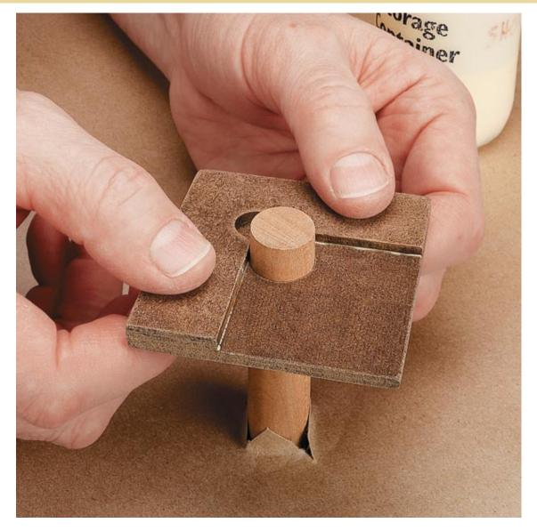
To make the bottom layer, I first drilled a relief hole where the fence edges intersect. This ensures that the faces of the fences will butt tight against the workpiece. Then it's a simple matter to cut the right angle. An auxiliary fence on your miter gauge makes this task easier. Then, to align the fences with the hole in the top layer, I used a dowel with the same diameter as the hole.
