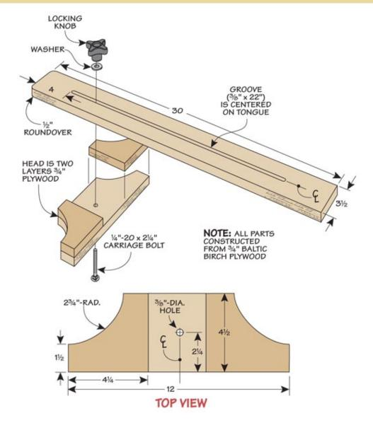
What makes the square so versatile is its sliding tongue design. As you can see in the photo and drawings, there's a long slot cut along the length of the tongue.
