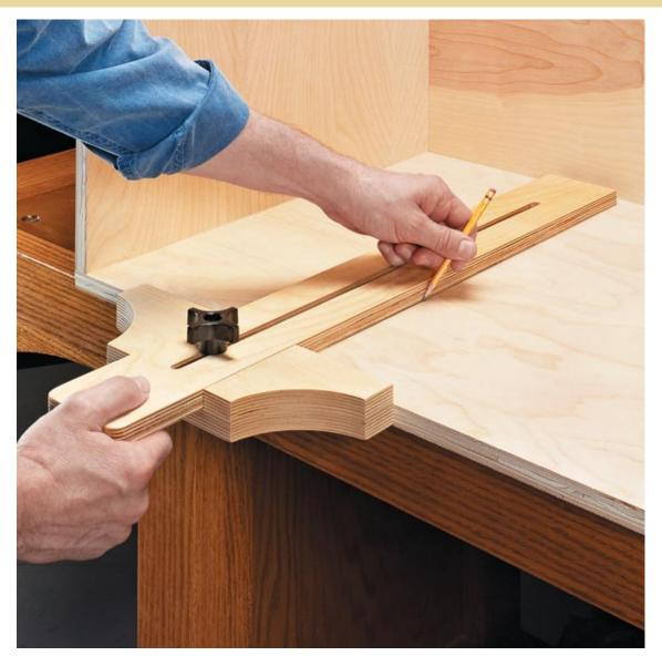
I've built quite a few cabinets over the years. And one of the challenges that always comes up is marking a straight line on the inside of the case for partitions or drawer slides. The problem is most store-bought squares are either too long to fit or too short to draw the line I need. The solution I came up with is an adjustable square. It's simple to build and works great. So well, in fact, that I use it all the time on all kinds of projects.
