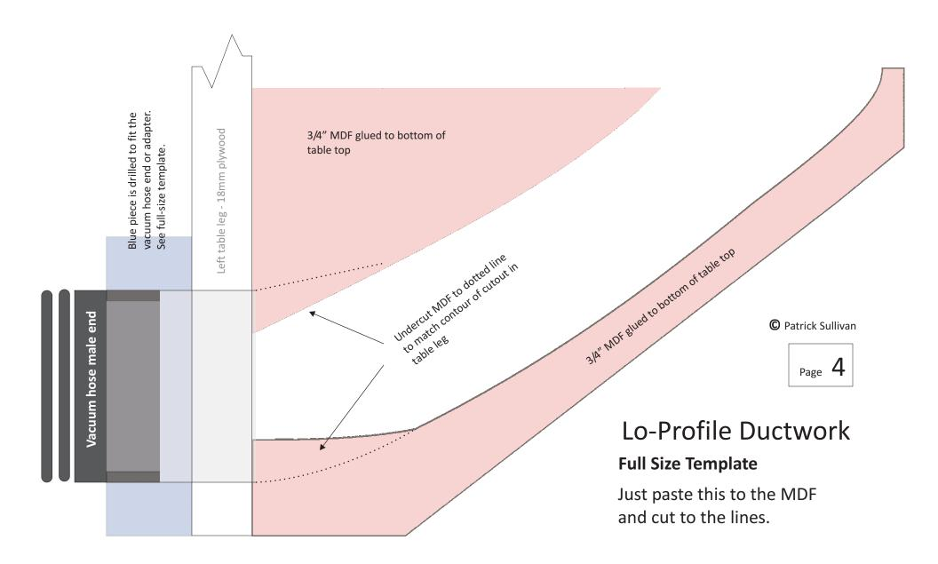
The thickness of the table top material might vary somewhat. 0.75" is the minimum. If you are using slightly thicker material, the only change you need to make is to adjust the height of the blue shape below to sit flush with the top. The hole shown is 2.25". However, it must fit your vacuum hose male end or adapter. These come in a variety of sizes.
