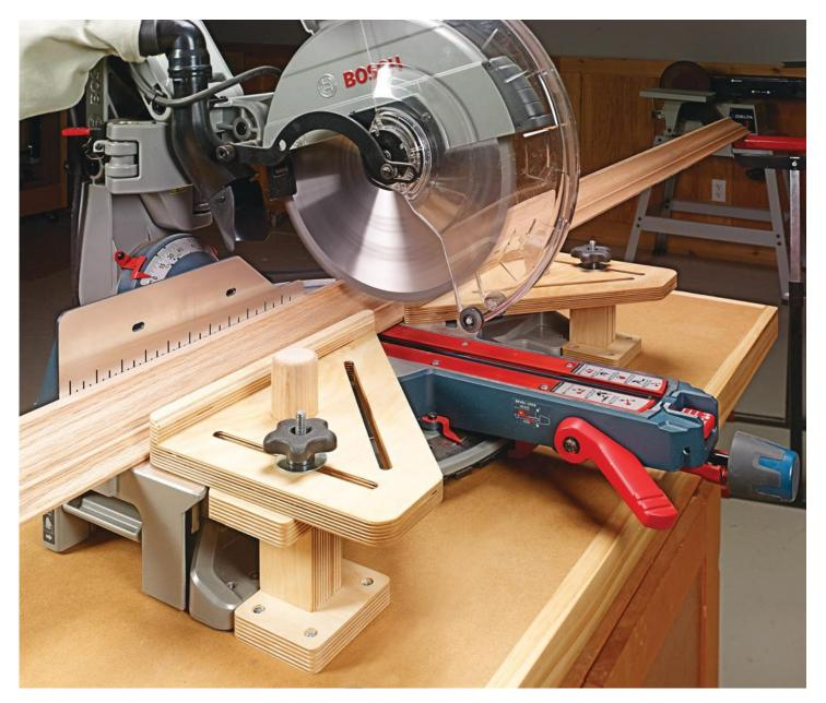
Using your hand to hold a workpiece against the fence of a miter saw can be a dangerous proposition, especially if the workpiece is small or needs to be held at an angle (like the crown molding shown above). To assist in situations like this, I designed this dual outrigger clamping system to use on my miter saw.
