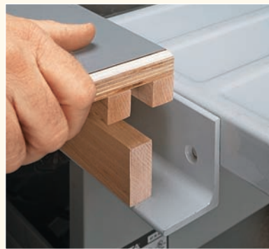
▲ A wood rail attached to the back of the table saw holds the outfeed support in place.
