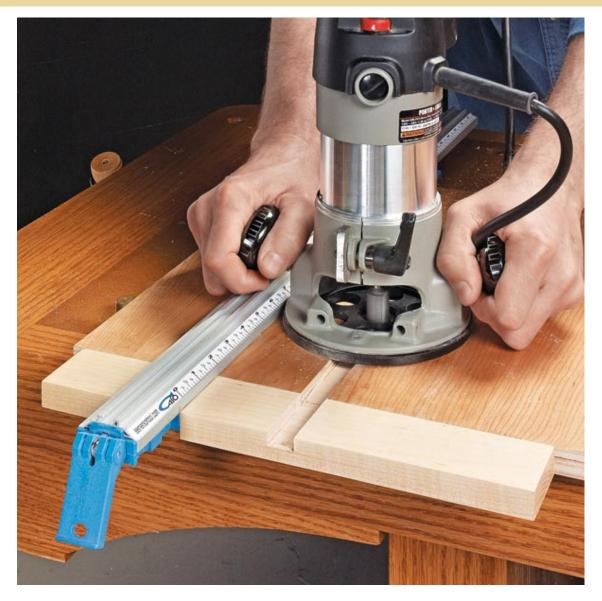
Using a straightedge guide is one of the best ways to rout dadoes and grooves. But trying to remember the offset distance from the outside edge of my router base to the cutting edge of my bit is a pain. Even when I do remember, I always feel a little uneasy, hoping that the cut will be in the right place. A quick and simple way to ensure accurate cuts every time is to attach an alignment board to your straightedge guide.
