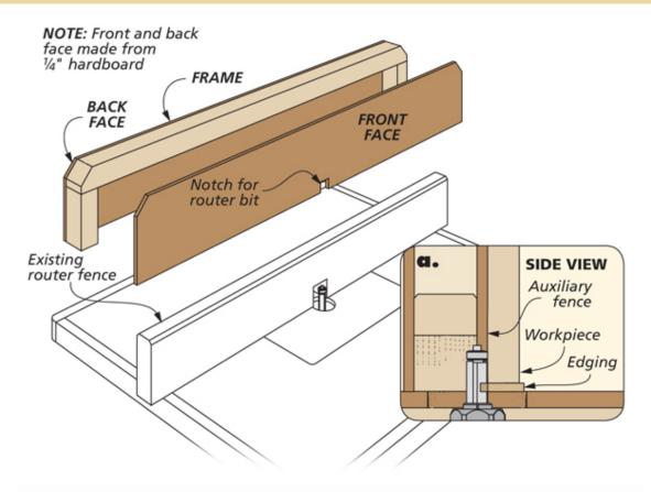
The secret behind this fence is that the front face of the fence is about 3/8" shy of resting on the table. This provides clearance to slide the wide edging under the face of the fence. To build the fence, I just glued all the layers shown in the drawing together after I cut a small opening on one face for the router bit.
