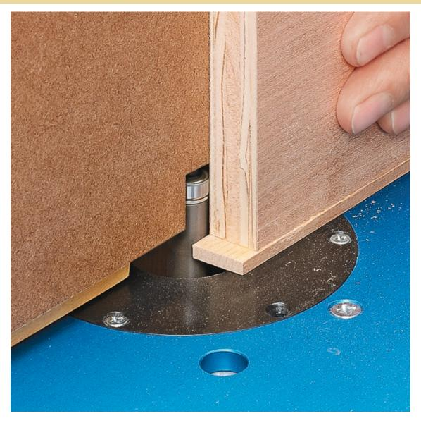
I needed a way to trim hardwood edging flush with plywood panels. Balancing a hand-held router on the edge isn't very stable. So instead, I turned to my router table. The solution is the tall router table fence you see here. The fence slips over my existing router table fence, so it's quick and simple to attach without using clamps or fasteners.
