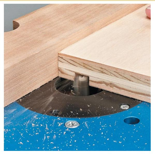
The straight edge can be used for routing grooves and dadoes. Just clamp the fence to the router table, positioning it away from the bit to properly locate the dado or groove in the workpiece.
