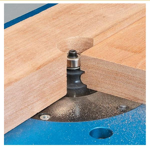
After ribbing Steve about his setup, I realized his "back-to-basics" approach deserved a closer look. As I said, his fence is nothing but a straightedged board with both edges are jointed straight. However one side is notched with a dado blade or Forstner bit to provide clearance for the router bit.
