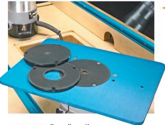
custom openings. Regardless of how the plate is made, most feature plastic reducer rings like the ones you see above. Having a set of reducer rings allows you to install (or customize) a ring to minimize the clearance around the bit. This makes for safer cuts and provides more
