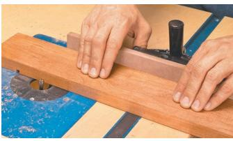
▲ Miter Track. Adding a miter track to your router table allows you to use other accessories, like the miter gauge and auxiliary fence you see here.
