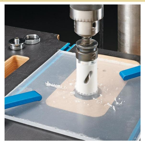
The process starts by cutting a square blank of  $^{1/4}$ - thick acrylic or polycarbonate plastic. Next, I worked on forming the stepped hole sized to fit the bushings and locking collar. This requires using a couple different hole saws.
