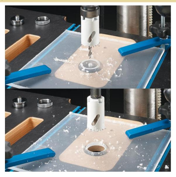
First, start with a 13/8"-dia. hole saw. This forms the "rabbet" or step for the flange around the bushing. The drilling depth should match or be slightly deeper than the flange thickness on the bushing.
