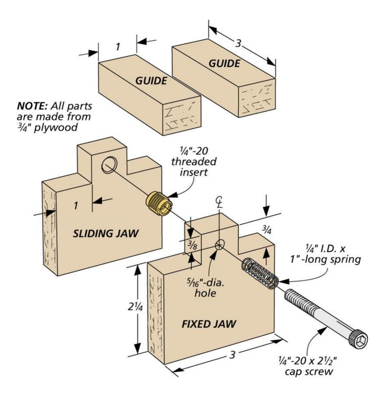
This saddle square is made from four plywood parts and some common hardware items. The fixed jaw has two guides <u>glued</u> in notches at the top corners. I cut the notches at the band saw. The rear, sliding jaw gets a <u>threaded insert</u> installed as shown above. A cap screw and small spring hold th sliding jaw in position. Depending on the spring's tension, this square will adjust to accommodate workpieces from 1/4" to 1 1/4" thick.
