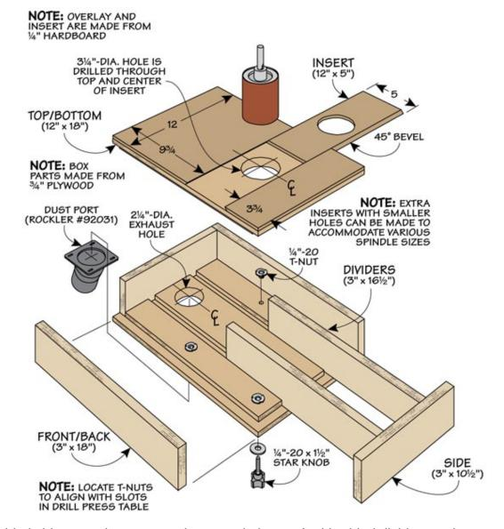
The table is big enough to support large workpieces. And I added dividers to the inside of the box to maximize airflow to the dust collector. Finally, to make positioning a workpiece easy, I added a smooth 1/4 hardboard overlay with interchangeable inserts.
