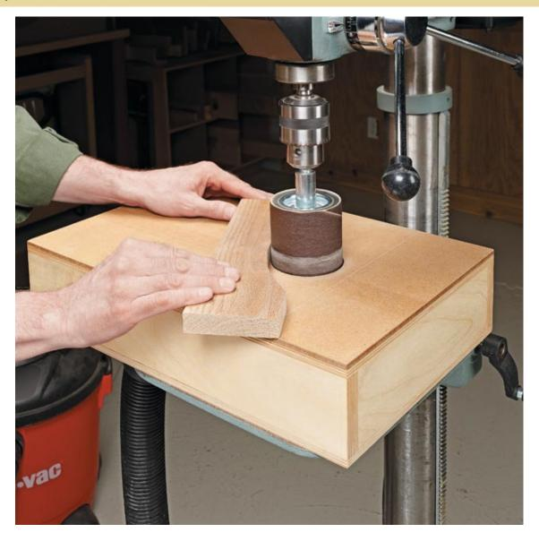
When it comes to sanding the inside of a curve on a workpiece, it's hard to beat a sanding drum in a drill press for speed and convenience. But the dust that results can be overwhelming. To keep the dust out of the air and my lungs, I came up with the table you see here.
