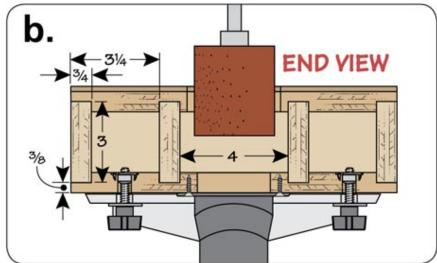
I made several inserts with different diameter holes to account for various sanding drums. The box extends off of one side of the drill press table to make room for a dust port on the bottom. T-nuts and studded knobs attach the table to the drill press.
