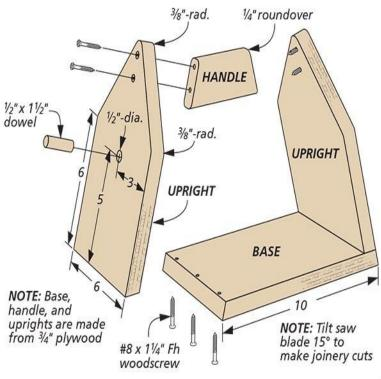
The saw blade caddy consists of four parts joined together with angled butt joints and screws. The center handle connects the uprights and makes the caddy easy to transport around the shop.
