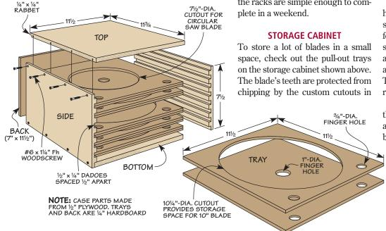
glue and screws. Once that's done, you can get started on making the trays that hold each saw blade.
