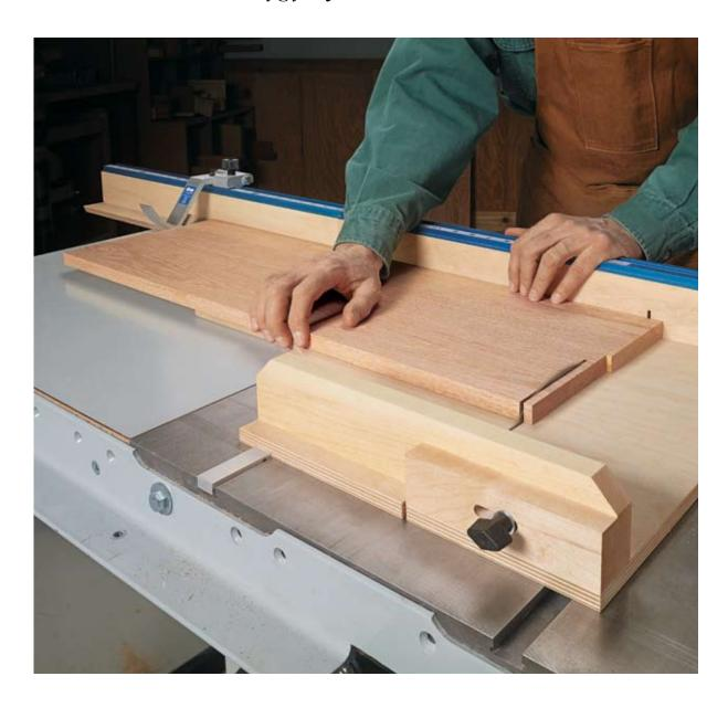
hen crosscutting on the table saw, I like the fool-proof accuracy a sled provides. This solid but lightweight sled makes cutting long or wide workpieces easy.
