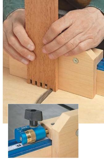
▲ **Box Joints.** You can easily turn the crosscut sled into a precise box joint jig with this commercial micro-adjuster.
