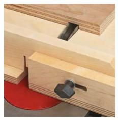
▲ Zero-Clearance Base. Whether you're making a simple crosscut or cutting dadoes, rabbets, or box joints, the adjustable base ensures less chipout.
