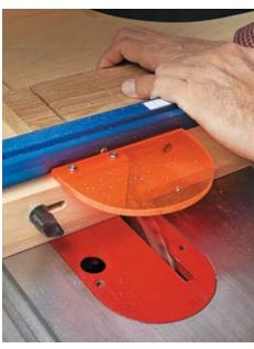
**Blade Guard.** The guard helps keep your fingers away from the spinning blade as it exits the sled.
