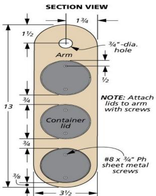
The swivel rack is a simple build. With the exception of the dowel and the PVC Spacers, the storage rack parts are all made from plywood. I made the top, bottom, and back first. A shallow hole in the top and bottom holds the dowel, and a couple rabbets are needed at the ends of the back. Next, cut the arms to size. Drill a hole in each arm for the dowel to pass through and use a couple screws to secure three lids to the underside of each arm.
