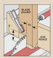
**The First Cut.** Using an auxiliary fence on your miter gauge, begin by forming the notches for the permanent fences in the blade guard.
