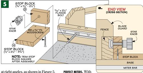
at right angles, as shown in Figure 5. You'll drill a hole in the back that's used to attach them to the fences. I made two of them so I could have one on each fence.
