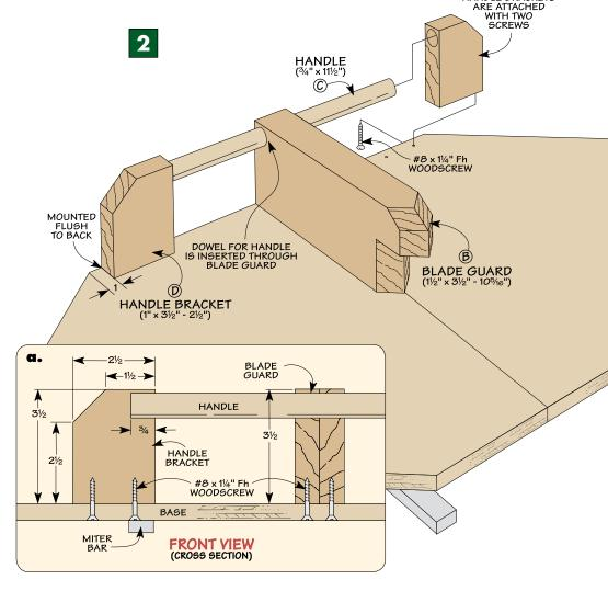
**READY FOR FENCES.** At this point, the base of the table saw sled is complete except for the two permanent fences and non-skid material. But before you move on to making the
