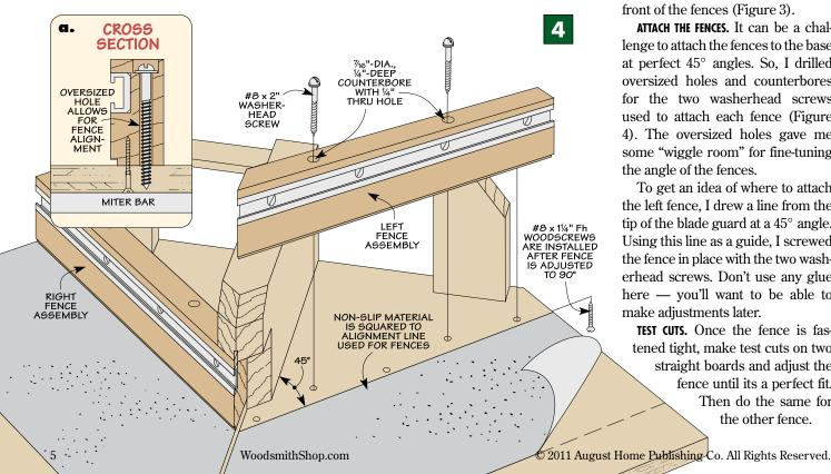
NON-SLIP SURFACE. Sometimes when I'm cutting miters, the workpiece has a tendency to "creep" as the saw blade starts to cut. To solve this problem, I found some non-skid material that is often used on stairs. As you can see in Figure 4, I aligned the material with the front face of the fence. You'll have some material hanging over the edge of the base to trim with a utility knife.
