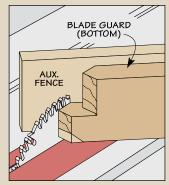
Forming the Nose. Then flip the guard over and make two 45° cuts. The point should be centered to help align the guard with the blade.
