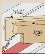
**Miter for the Fences.** Rotate your miter gauge 45° to complete the notches where the fences will rest. Make two cuts to center the point.
