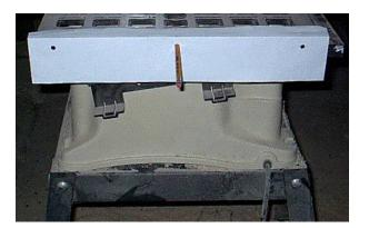
Take a piece of plain paper to use as a template and fold it so that the paper will fit over all three holes on the side of your table saw (fold the paper so that the "L" shape dimension is: 1/2" x 3"); hang the paper over the edge of the table covering the three holes on the side of the table top; measure and mark the center of the Center Hole on the 1/2" lip of the paper; mark all
