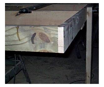
Select two  $1 \times 4 \times 8'$  and lay them on edge on a flat service/floor; select two pieces of the  $1 \times 4 \times 22''$  and lay them on edge, one at each end, and screw them together (use a speed square to ensure all angles are square).
