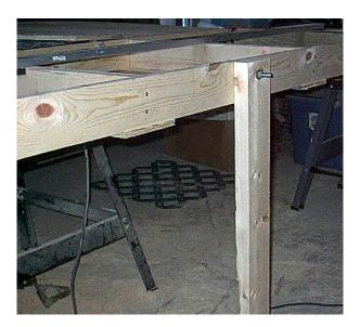
After completing the second Extension, lift them up into position; tighten the Support Leg into position; attach the Table Extension to the saw with the 3/16" bolts, washers, and wing nuts.
