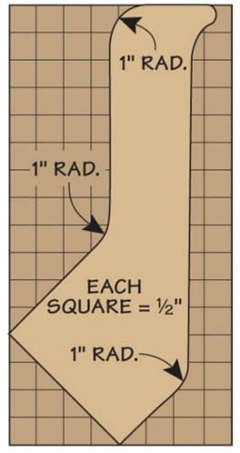
Use this pattern to create the shape of the handle. After cutting it out at the band saw or with a jig saw, you can soften the edges with files and sandpaper.
