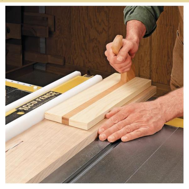
When I'm ripping stock at my table saw, I like to keep downward pressure on the workpiece as I'm making the cut. The push block you see here is just the ticket.
