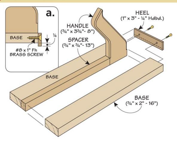
The sturdy handle and long base make it easy to rip stock of any size. And the brass screws holding the heel mean that it can be replaced after being chewed up from repeated use.
