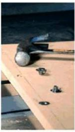
T-nuts are easy to install using a hammer if you drilled your holes correctly in your base. Drill the  $\frac{3}{4}$ "-diameter hole for the flange using a Forstner bit. Then use the hole left by the bit's spur to center the  $\frac{3}{4}$ 16" bit for the through-hole.
