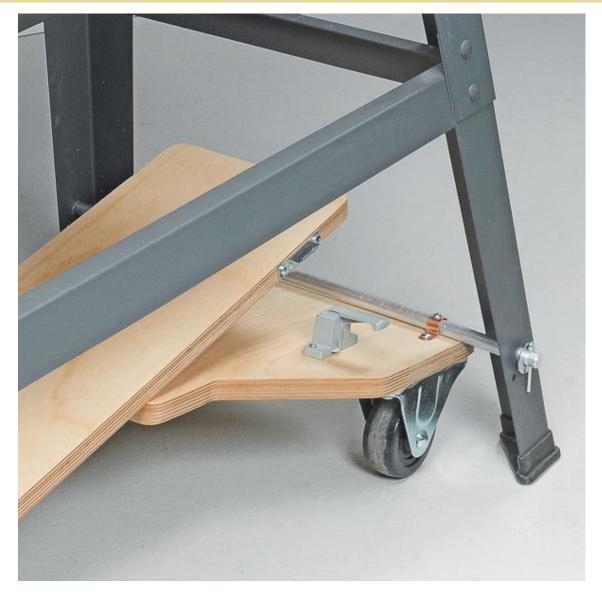
With the rods in place, you can attach each wing to the rod with a pair of straps. I drilled and installed a screw through the rod to keep the wings from slipping side-to-side. Finally, I installed a screen door latch to secure the wings in the "mobile" position when moving the tool. Simply tapping the latch with your toe releases the wings to lower the stand to the floor.
