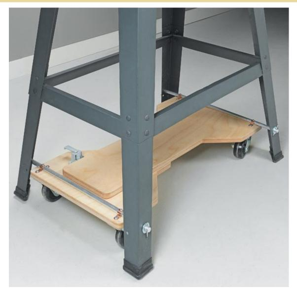
My shop is small, so mobile bases for my tools are a must. The problem with most commercial bases is that the casters are outside of the tool stand and it's easy to trip over them. The compact, shop-made version you see here places the casters on the inside of the stand. And what's more, the design is easy to operate with light foot pressure. Plus, it uses common, inexpensive hardware.
