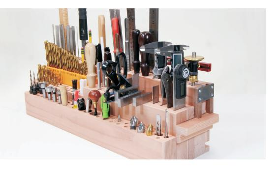
On the next two pages you will find the overall dimensions of the case I built. However, most of the dimensions are very arbitrary and flexible. I built this in the USA, using a redwood "2x6", a misleading term that means it is 1.5 inches thick, and 5.5 inches wide. If building in metric, then obviously choose dimensions that fit the wood you have available.
