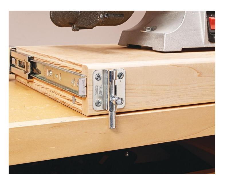
To hold the platform in place while in use, I installed a couple of barrel bolts on the front.
