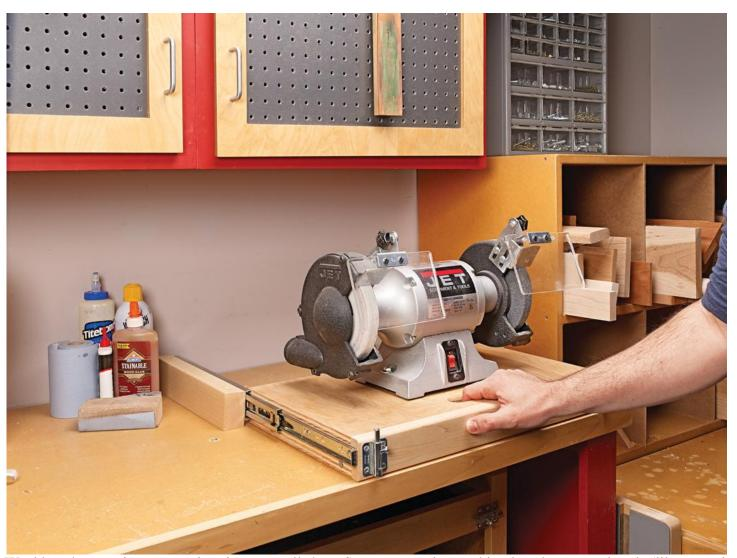
Workbench space is at a premium in my small shop. So permanently attaching bench-mounted tools (like my grinder) in a convenient position at the front edge of the bench is not an option. Instead, I made a simple pull-out platform that allows me to slide my grinder to the front edge of the workbench when I need it.
