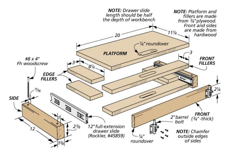
The platform is just a few layers of plywood assembled with glue. A hardwood front covers the plywood edges. A pair of full-extension drawer slides are mounted to the sides and platform. The sides are screwed to the workbench.
