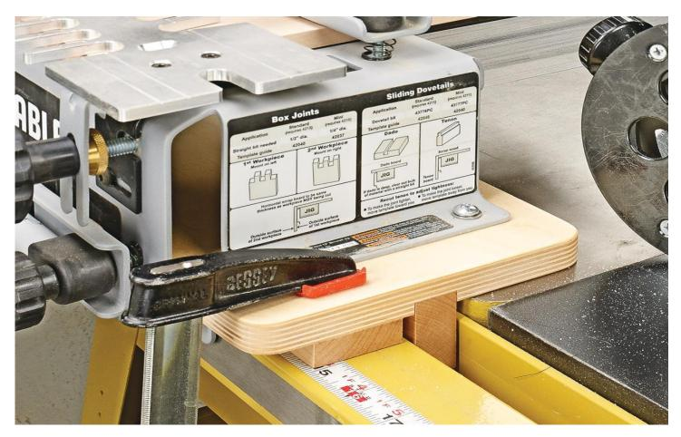
The whole assembly is then clamped to the fence rail. It's easy to customize these mounts for other bench top tools.
