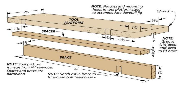
My table saw has a gap between the L-shaped mounting bracket and the rail that the fence rides on. I sized a board to fit in that gap and then attached it to a platform that's sized to fit my dovetail jig. Another board attached to the bottom of the platform acts as a spacer to bring the platform level with the top of the saw table.
