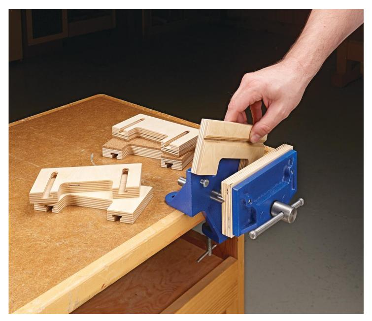
I have used a 6" clamp-on bench vise in my shop for many jobs. When it was new I installed some simple wood jaw faces in the vise to make it easier to use for woodworking. But over time, these wood faces had become nicked, scarred, and encrusted with glue. Needing some new faces, I decided it would be useful to make a few different styles for various tasks. I also wanted to make them so they would be easy to switch out. What I decided on is the design you see above.
