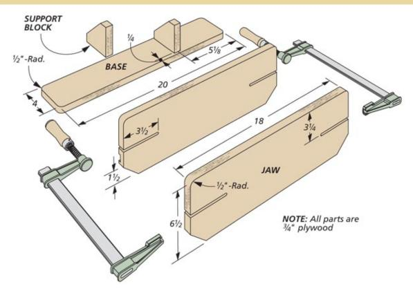
The vise consists of two jaws with slots sized to accept my clamps. The rear jaw attaches to a base that can be secured to almost any worksurface.
