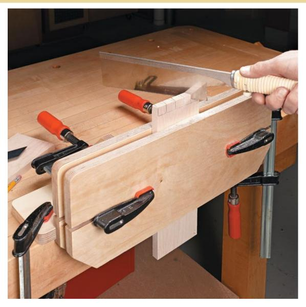
I've always found it helpful to have more than one vise in my shop. This notion inspired the simple small parts vise you see above. It's based on a centuries-old woodworking vise design, but I modified it to be made out of plywood and a few clamps. It elevates the workpiece, which I've found to be helpful for my back when working in the shop.
