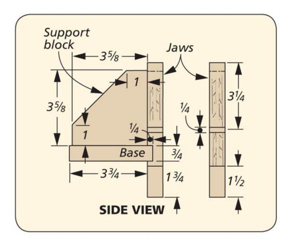
The rear jaw has a groove cut in the back face to make a solid connection to the base. Two support blocks keep the rear jaw square with the base. The rear jaw is glued to the base to complete the assembly.
