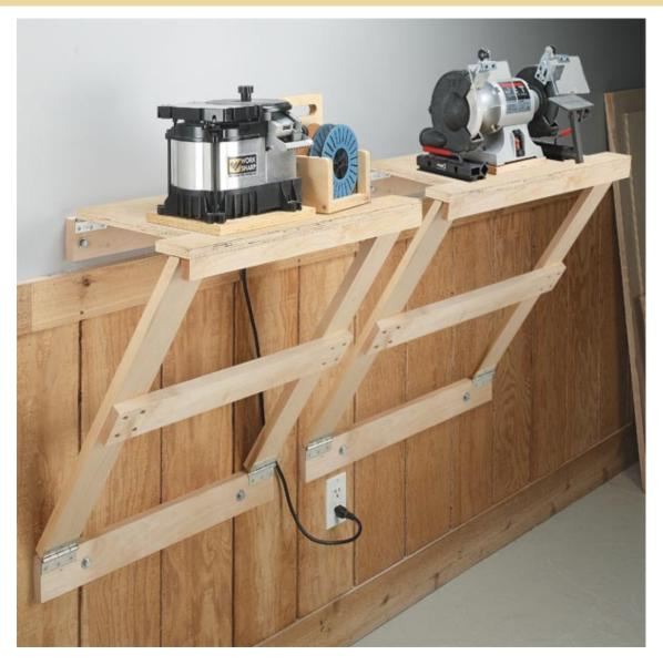
Having my workshop in the garage means I can't always leave things set up. My solution is a set of hinged, fold-up workstations. You can mount the tools permanently or make them easy to remove.
